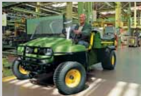
TE Gators can be used indoors due to low engine emissions and quiet operation.
