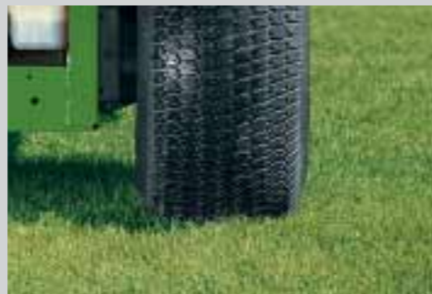
High-flotation tyres allow both Gators to work hard without scuffing the turf.
