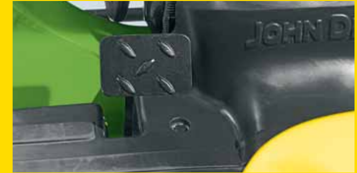
Two-stage differential lock and brake. Gain traction and stability, even on rough terrain. When pushing down more, the brake will safely stop the tractor.
