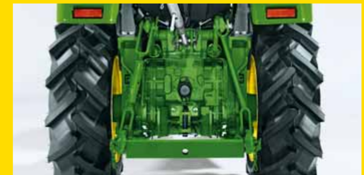
High rear hitch lift capacity. With 600 kg lift capacity there is almost no limit to handle attachments.
