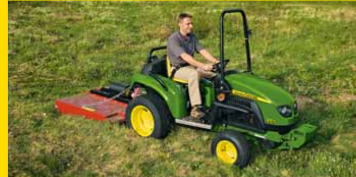
Standard foldable mid-mount ROPS. Leave it up for safety or fold it down to get the clearance you need.
